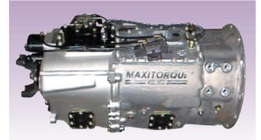
on or on/off highway. The low forward ratio is 13.44:1 and top gear is .71:1 overdrive for highway cruising. PTOs can be driven from both fixed and speed dependent mounts on all models. (For applications which require backing control and a slow 28.98:1 reverse ratio, refer to the data sheet on the T-313LR21.)
