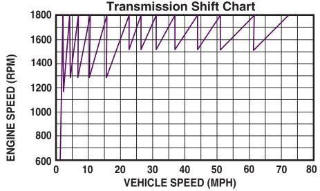
T-31321 w/1800 RPM ENGINE, REAR RATIO 4.17 AND 11R22.5 TIRES (BASED ON 504 TIRE REVS PER MILE)
