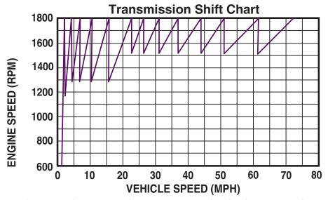
T-313 w/1800 RPM ENGINE, REAR RATIO 4.17 AND 11R22.5 TIRES (BASED ON 504 TIRE REVS PER MILE)
