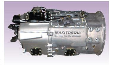
PTOs can be driven from both fixed and speed dependent mounts on all models. (For applications which require backing control, the LR model features a slow 28.98:1 reverse ratio.)
